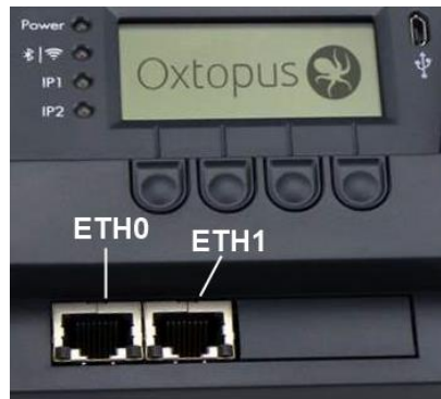
Figure 2 Ethernet Connectors Eth0 and Eth1
