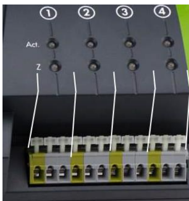
Figure 9 Wired connection TP/FT10 CEA_709.1
